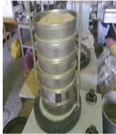
Sieve analysis of mango kernel powder
