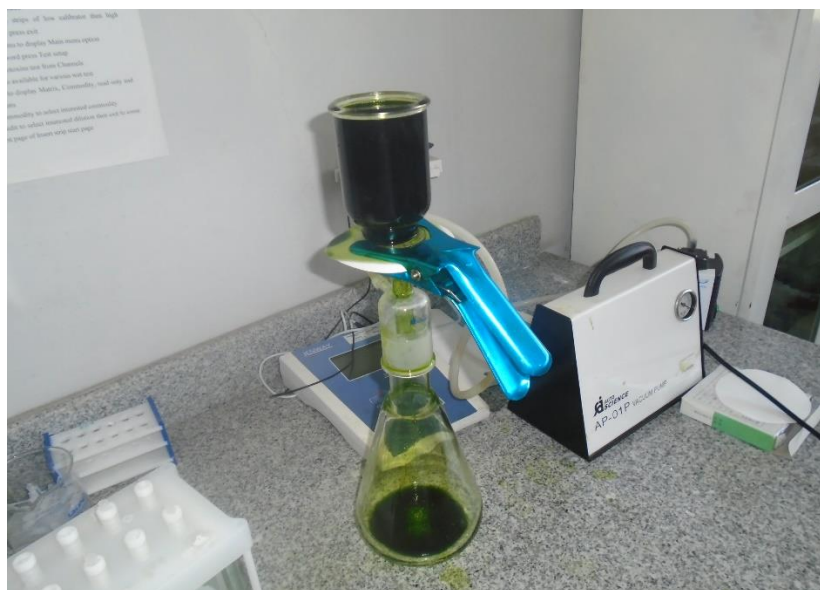
Figure 4: Filtration of Ricinus communis Linn crude extracts via Whatman no.1 paper by filtration apparatus.
