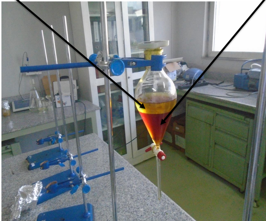
Figure 6: Solvent fractionation of crude methanol extract of Ricinus communis Linn leaf in the separatory funnel.
