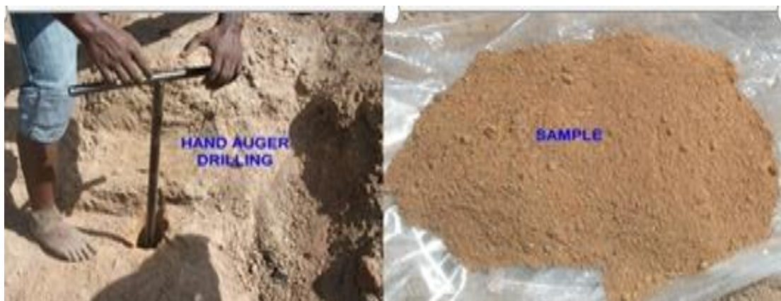
Figure 4.1.1 representative sample of cement raw material
