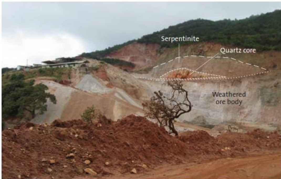
Fig 3.4.3 Weathered tantalum ore body (white) underlying talc-tremolite schists and serpentines. The quartz core is standing out
