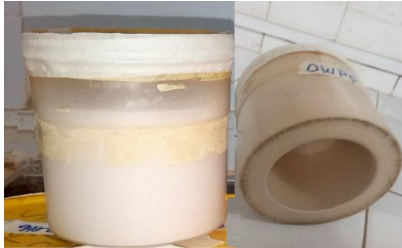
Figure 3.1.6-1: Sample filled in a geometrical beaker and sealed
