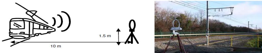
Figure 2.16 On site measurement of the electromagnetic radiation of the train [13]
