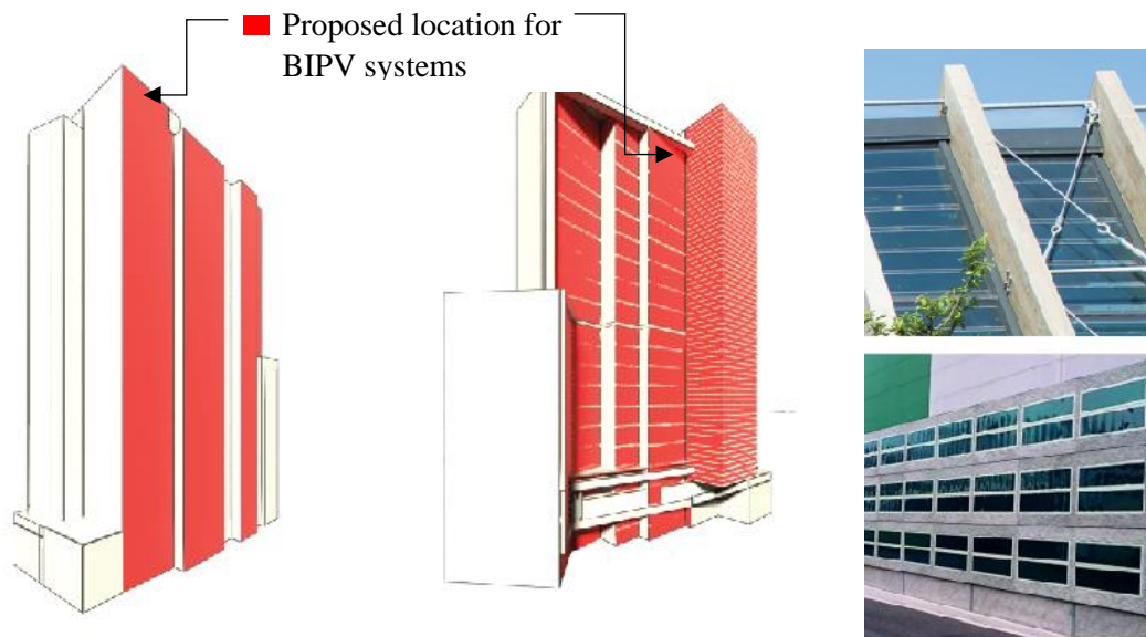
Figure 4.23 – Proposed location for the BIPV system (from Hidassie Telecom HQ project archives)
