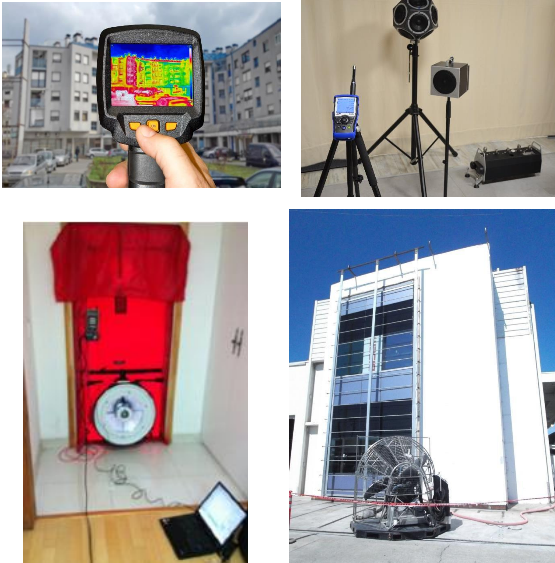
Figure 2.1 – Thermography (top left) (TSI Energy Solutions, n.d.), Acoustics measurement (top right) (Building acoustics measurement set, n.d.), Fan pressurization test (bottom left) (Kim et al., 2012), curtain wall performance mock-up test (bottom right) (Carbary et al., 2014)
