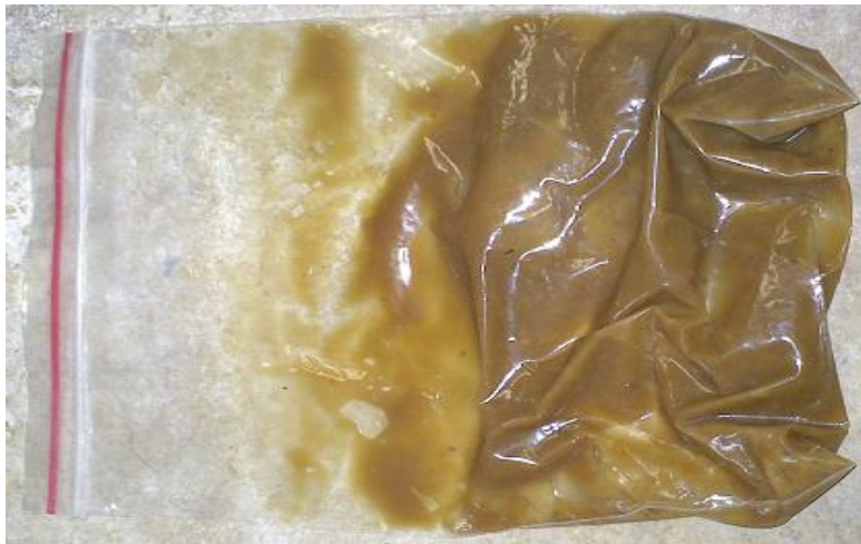
Fig.3.12 Paste of protease prepared by spray drying for dehairing skins and hides
