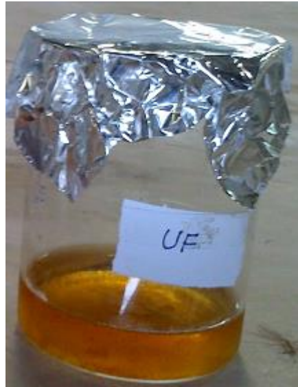
Fig.3.11 Sample of protease prepared for dehairing skins and hides by U F
