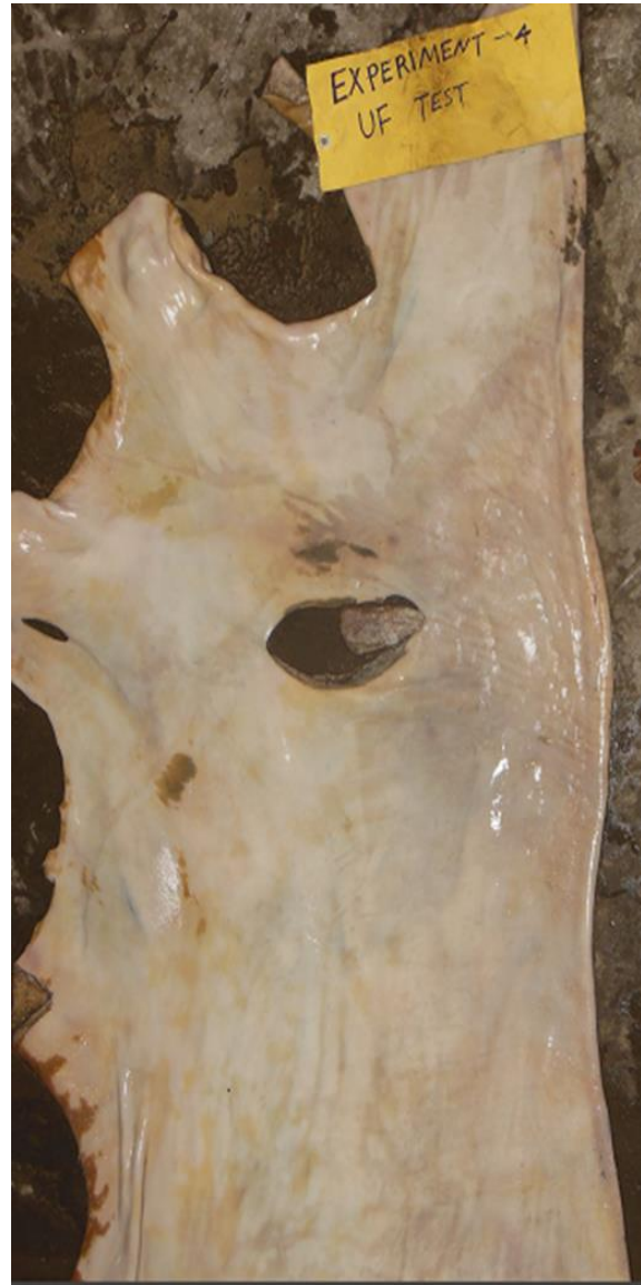
Fig.4.16b Cow hide after unhairing
