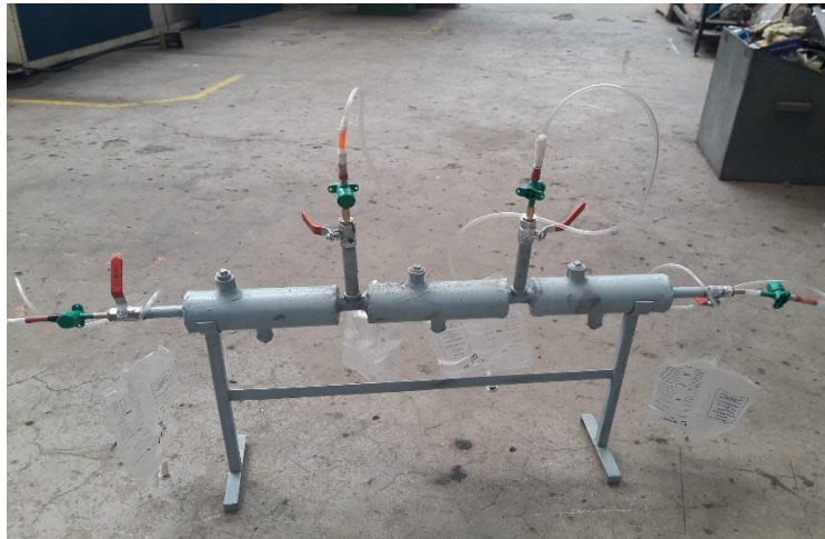
Fig 3.11 Raw biogas scrubbing set up
