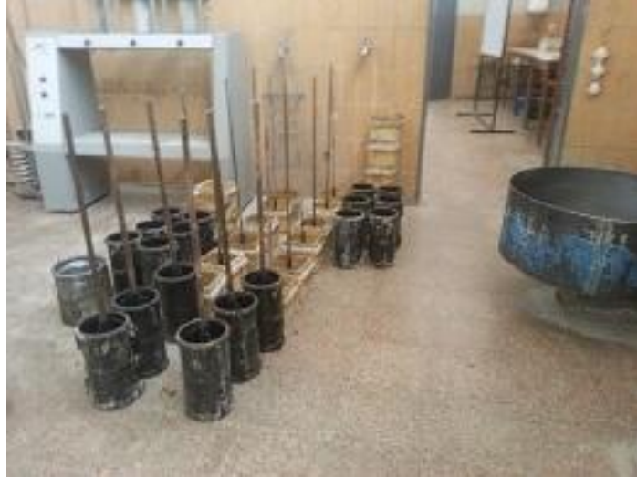
Fig. 3.8 Reinforcement placed in form work
