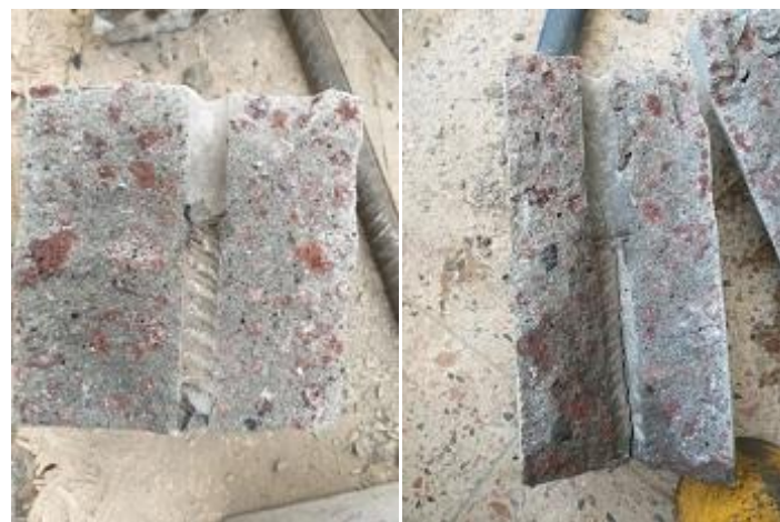
Fig. 4.2 Typical failure mode and surface of Pull-out specimens (Sc-Sa mix) after testing
