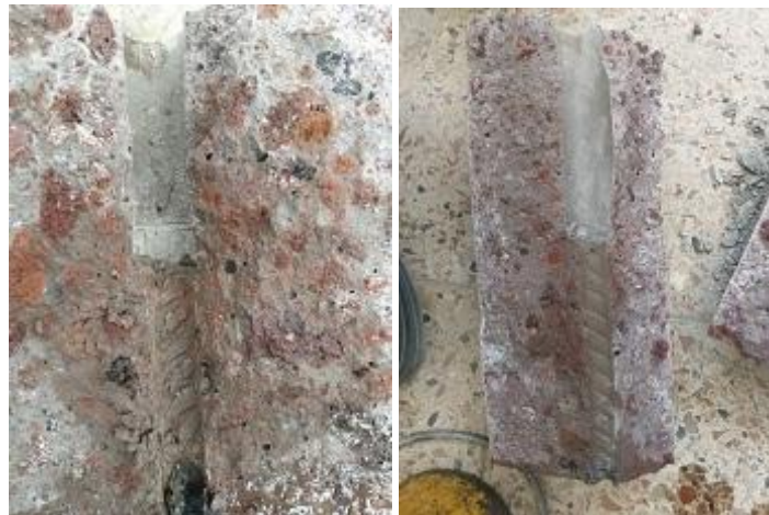
Fig. 4.1 Typical failure mode and surface of Pull-out specimens (Sc-Sc mix) after testing
