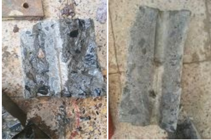
Fig. 4.3 Typical failure mode and surface of Pull-out specimens (N mix) after testing
