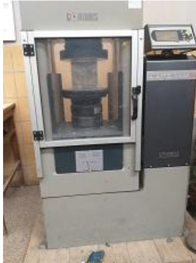
Fig. 3.4 Compressive Strength testing machine
