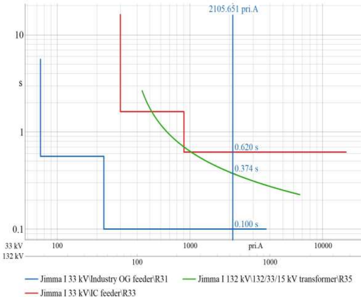
Figure 4.1: Time-Overcurrent curve as well as operating time responses for relays R31, R33, and R35 with a 3-phase short-circuit fault current of 2.106 kA on distribution feeder.
