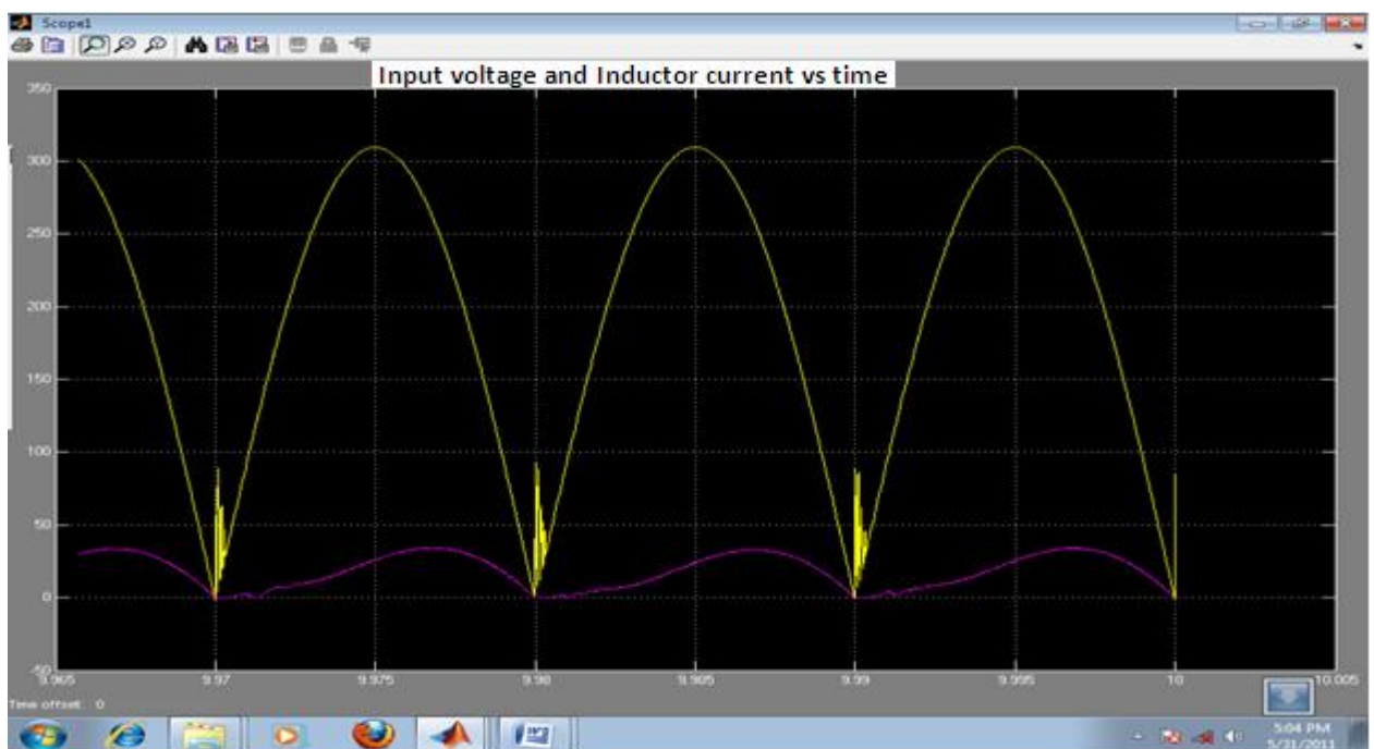
Figure 5.14: The rectified input voltage (upper) and inductor current (lower) of the current mode controlled converter
