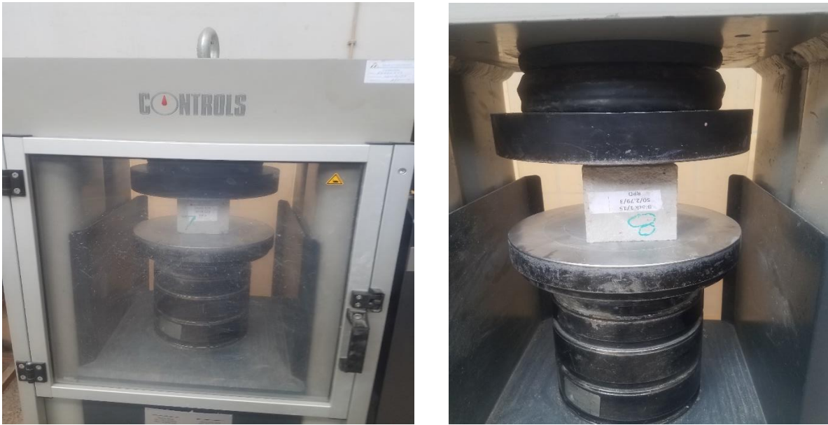
Fig. 3 measuring the compressive strength of the concrete cube samples using Automatic compressive strength measuring machine
