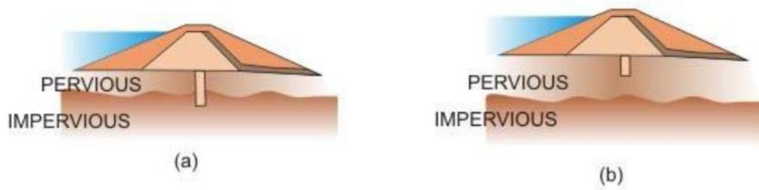
Fig. 2.6 Concrete diaphragm; (a) Complete (b) Partial
