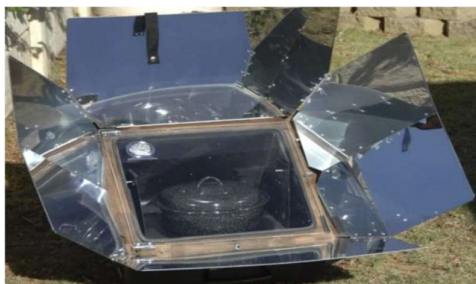
Figure 2.2: Panel Solar Cooker [17]
