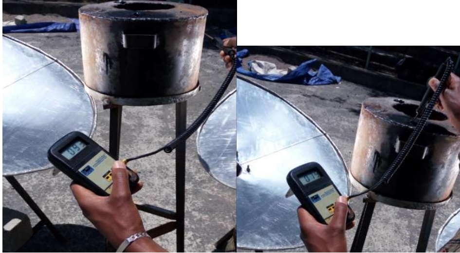
a. Measuring temperature of absorber surface b. measuring temperature of used engine Oil
