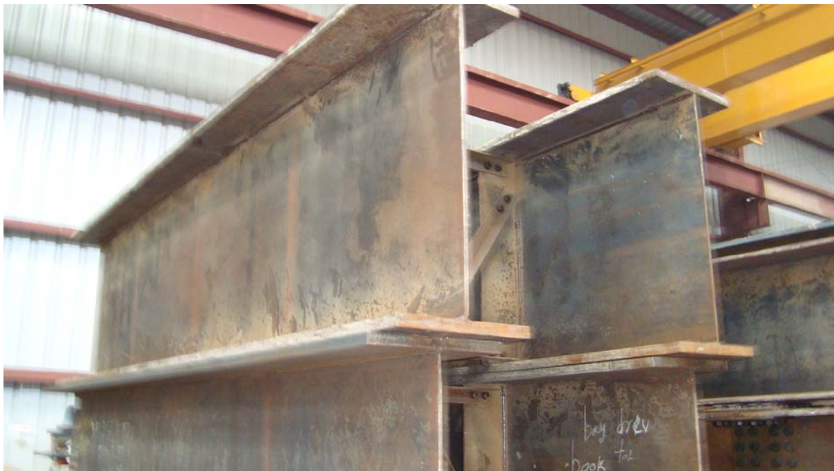
Plate 3.1: Welded plate girders of I section ready to be dispatched to rail way site for steel bridge.
