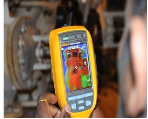
Figure 4-2 Temperature measurement on the steam header
