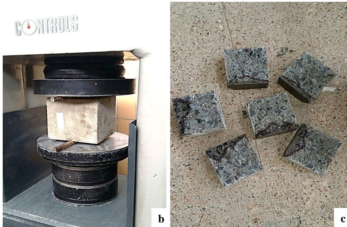
Figure 4-6: Water penetration test setup a) Test setup b) Splitting process c) Marked Specimen after splitting
