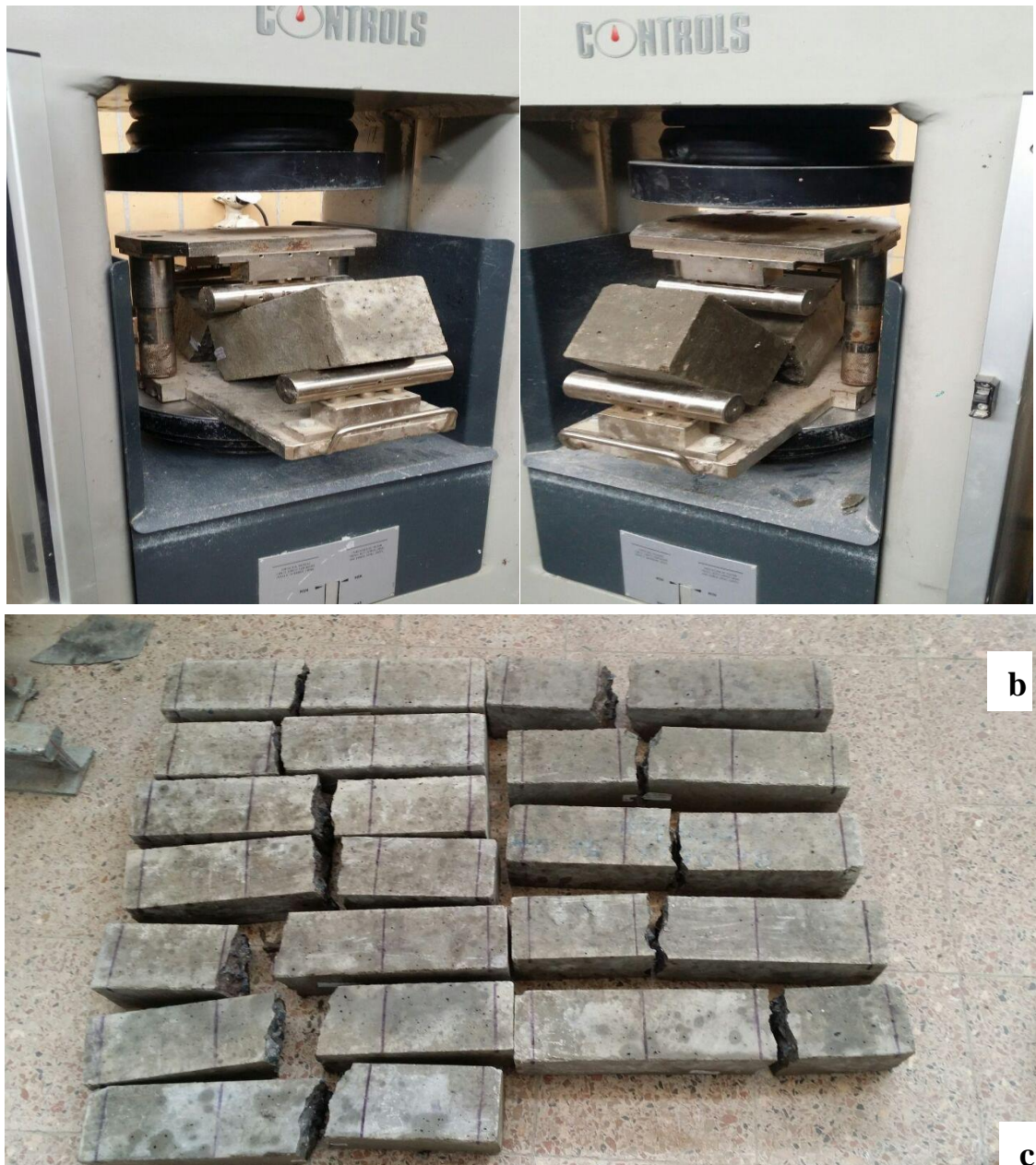
Figure 4-5: Flexural strength test setup a) Marked test specimen b) Specimen under test c) Specimen after test
