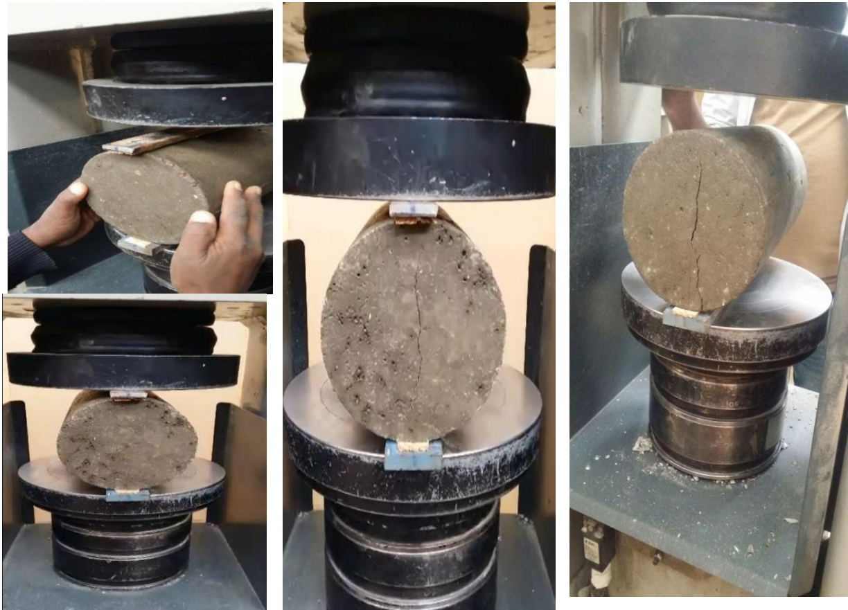
Figure 4-4: Splitting tensile strength test setup
