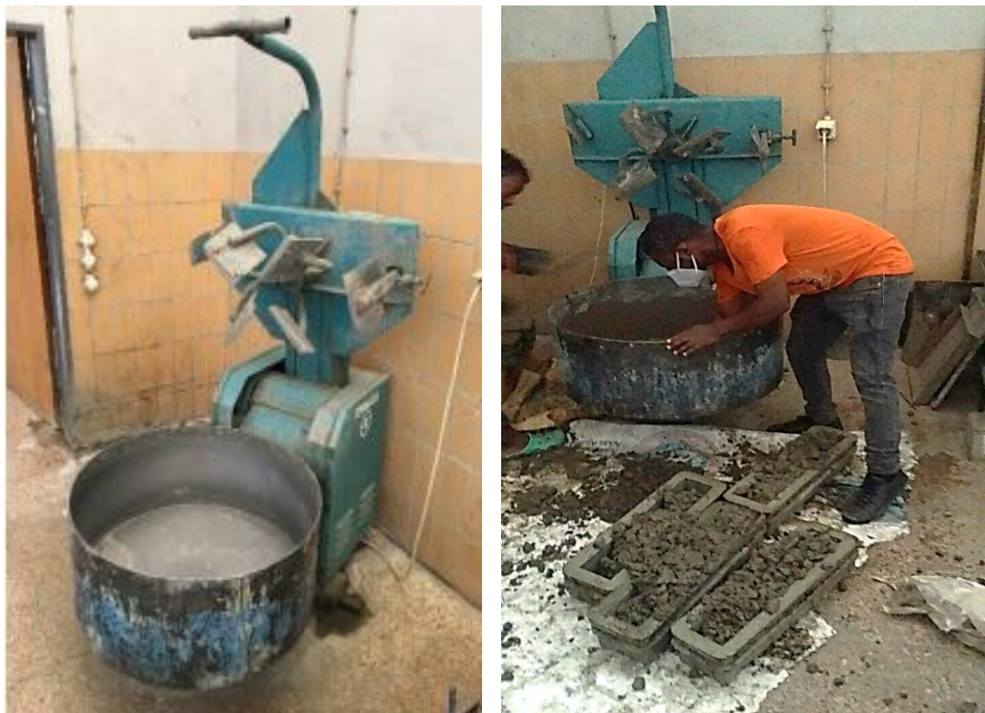
Figure 4-1: Concrete Mixing and Molding at the Laboratory
