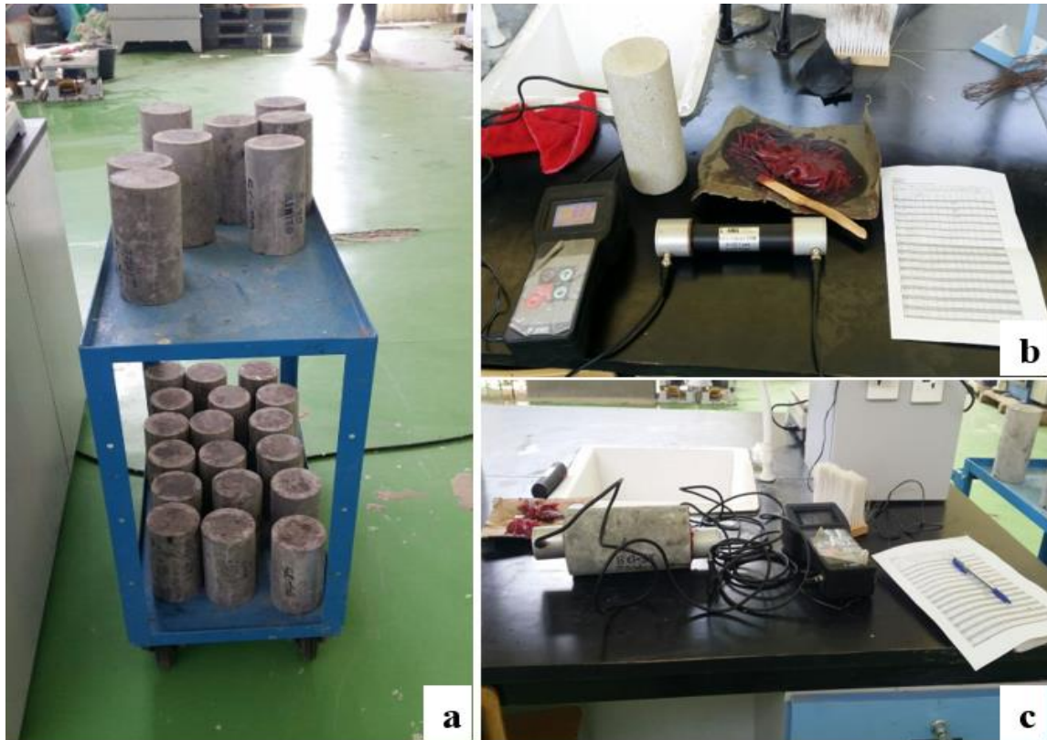
Figure 4-7: Ultrasonic Pulse velocity test setup a) Test specimens b) Instrument calibration c) Testing specimens
