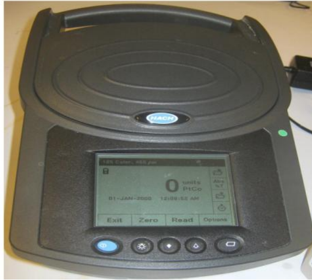
Figure 3.5: color measurement by using HACH model Spectrophotometer
