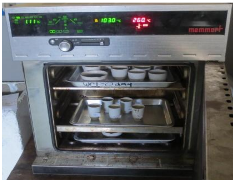
Figure 3.7: Wastewater samples in the oven for TS and TDS analysis.
