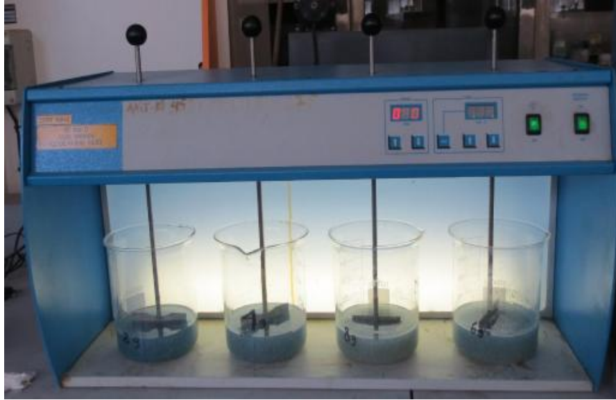
Figure 3.4: A jar test apparatus used for treatment of textile wastewater in coagulation
