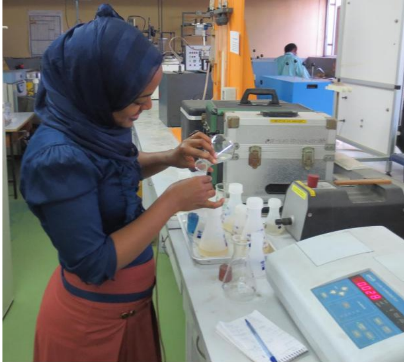
Figure 3.6: wastewater turbidity test by using HACH Turbidimeter
