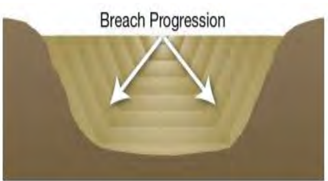
Figure 2.4: Overtopping trapezoidal breach progression
