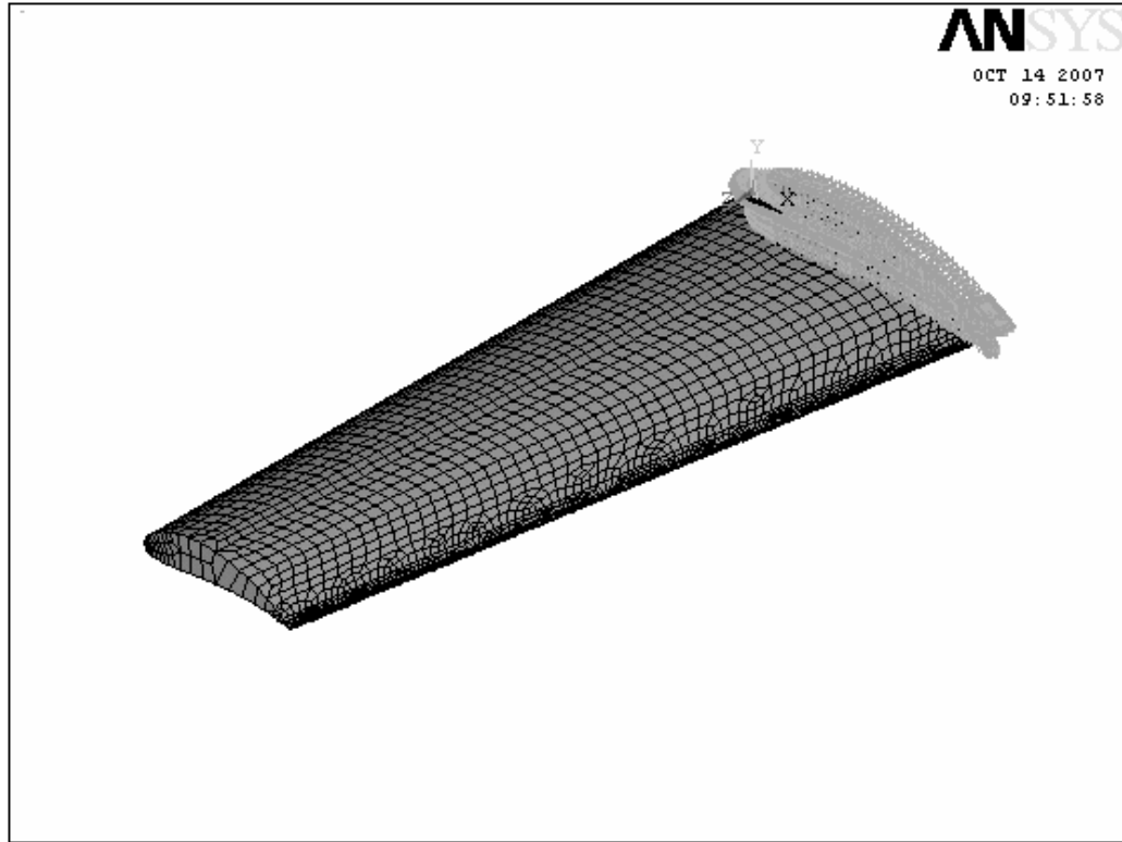
Figure 5.6 F.E Model with the boundary condition(subsonic wing)
