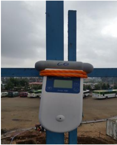
Figure 3: (a) Sampling of air pollutant gas matter
