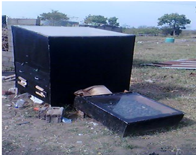
Figure 2.1. Passive solar incubator [18]
