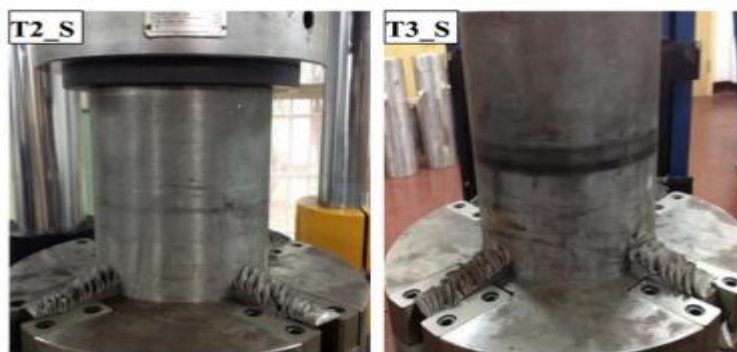
Figure 13 Deformation of steel tube during quasi-static test [17]
