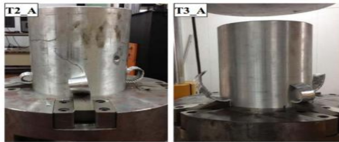
Figure 12 Deformation of aluminum tube during quasi-static test [17]
