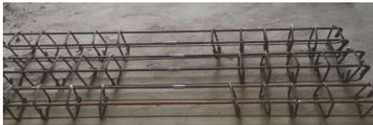
Figure 3-5: Reinforcement Arrangement in the Specimen Beam
