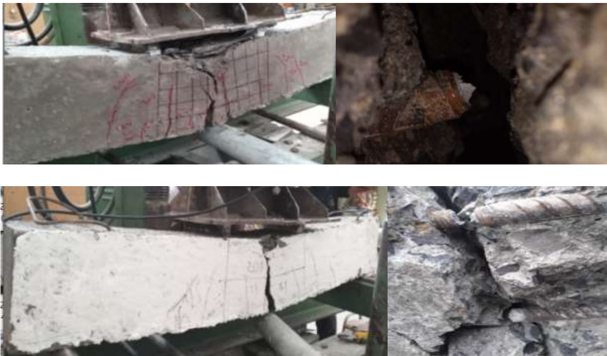
Figure 4-5: Mode of Failure for CIB-2 beams
