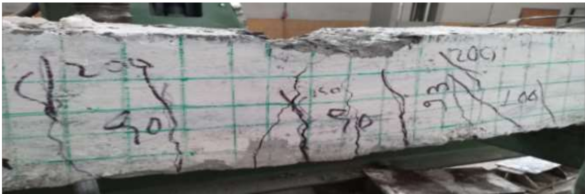
Figure 4-3: Mode of Failure of Control Beam Specimen
