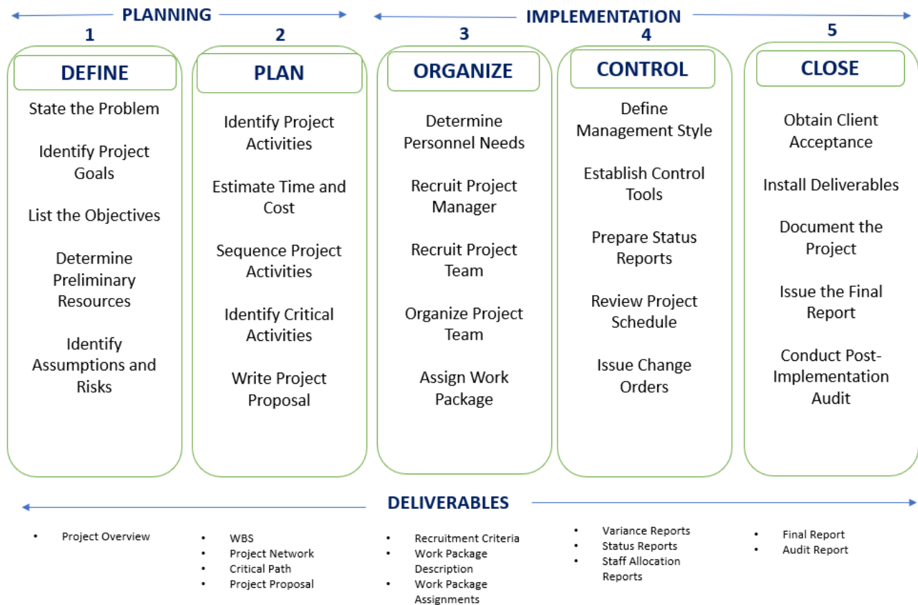
Fig. 2.4 - The five phases and 25 action steps of the project management life cycle
