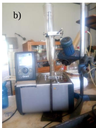
Figure 3-5 a) Centrifugation b) Rotary evaporator c) DMA 4100 M (digital density meter)
