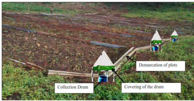
Figure 4. Surface runoff volume collection from the four tillage systems in the study sites.
