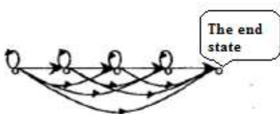
Figure 2.1: The structure of Left –to-Right HMM with state skipping.
