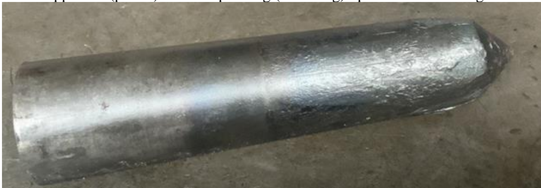
A: 1.4 the forged hot pickaxe at the moment of end forging operation
