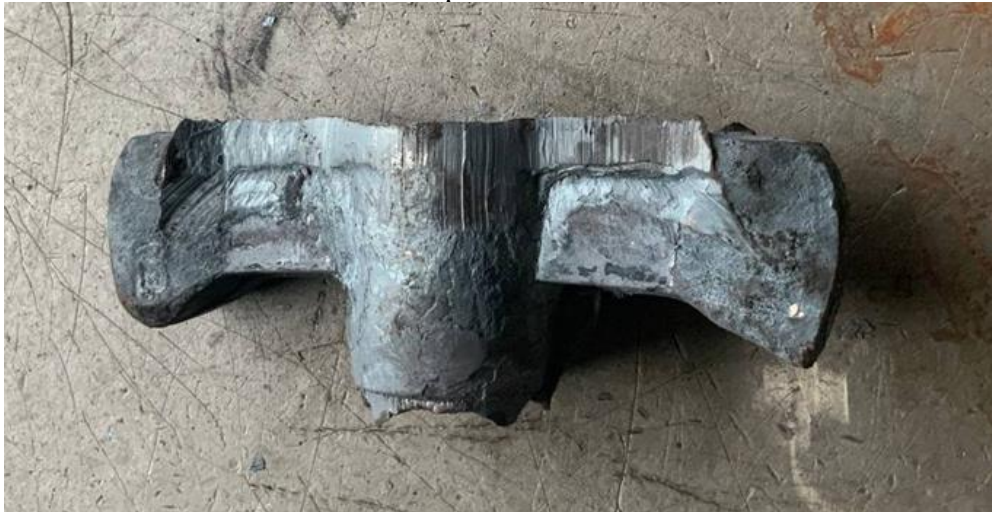
A: 1.5 trimmed and semi-finished pickaxes
