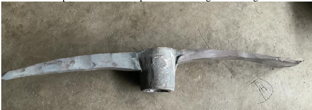
A: 1.6 finished pickaxe and the shape modified using hammering machine.
