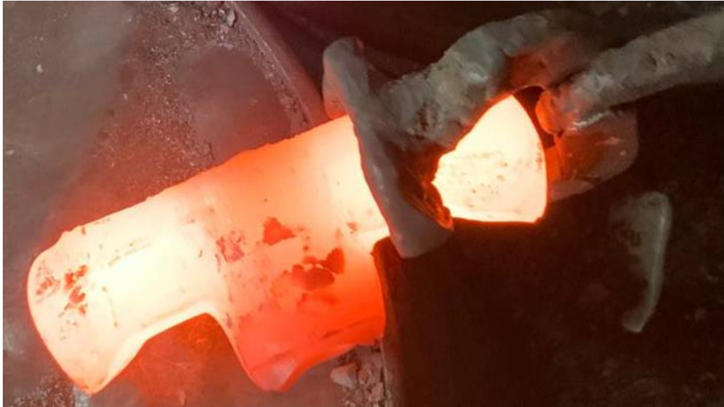
A: 1.5 trimmed and semi-finished pickaxes
