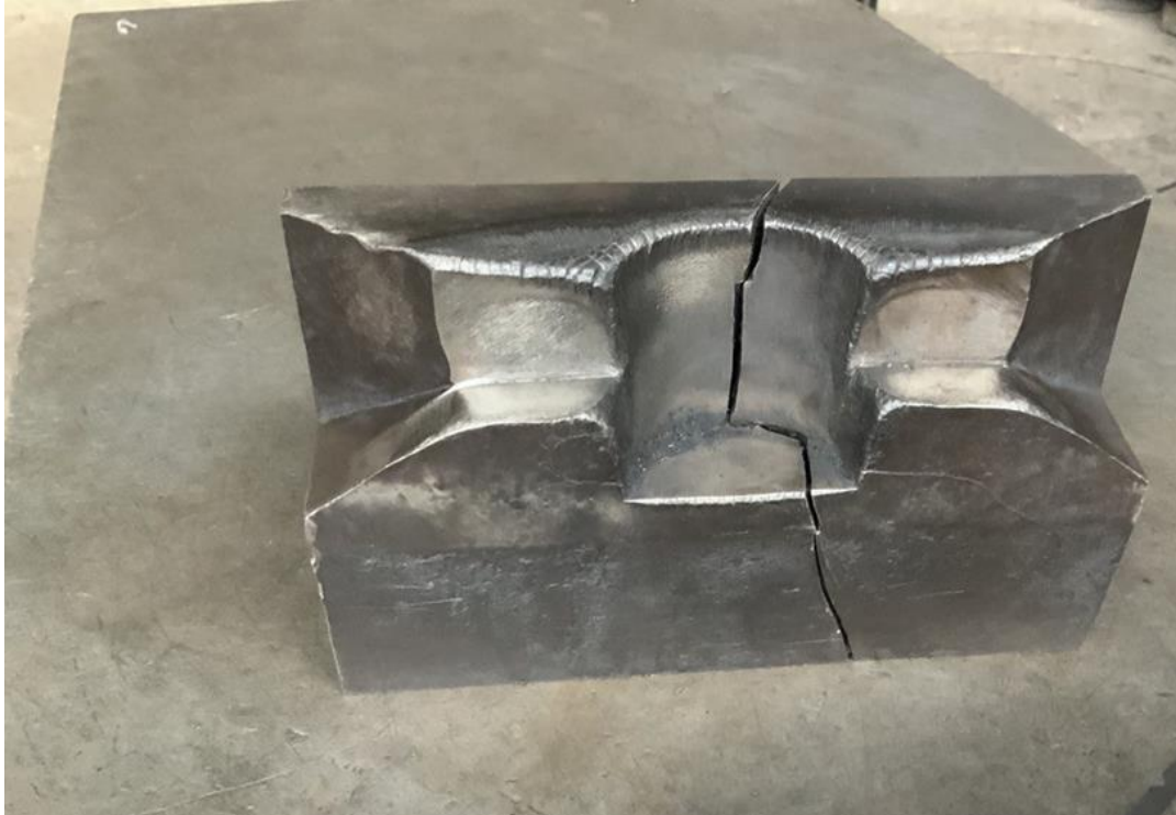
A: 1.3 upper die (punch) used for piercing (indenting) operation for making hole.
