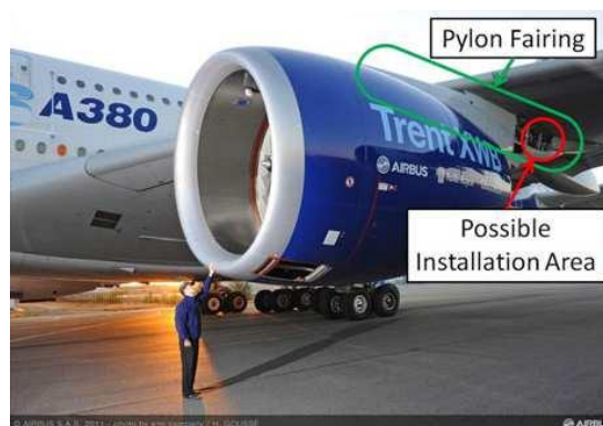
Figure 2-24: Opportune spot for placing of TEG on the pylon fairing of Airbus A380 [13]
