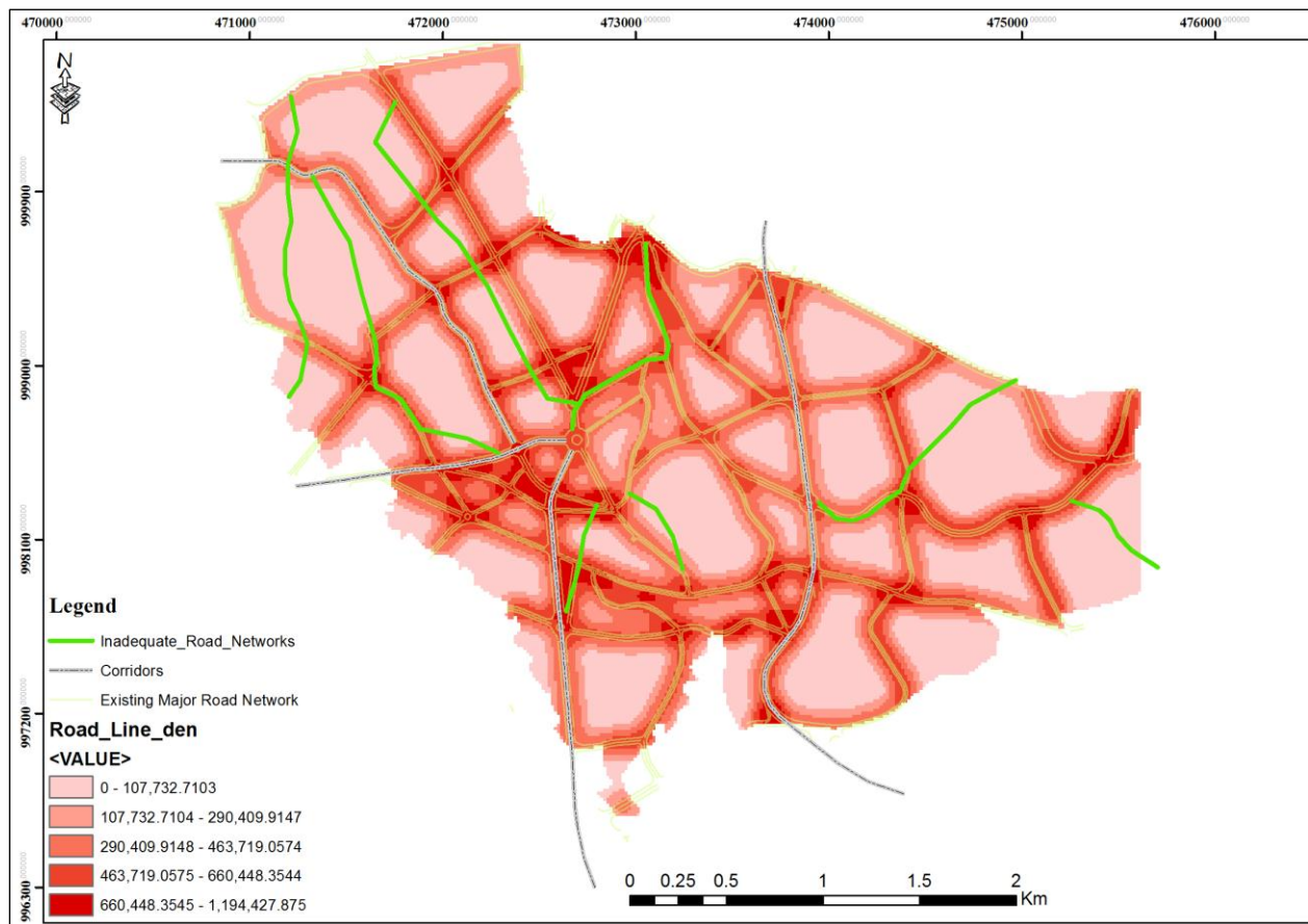
Figure 6.3: Map of Inadequate Road Networks and Value of Road Line Density
