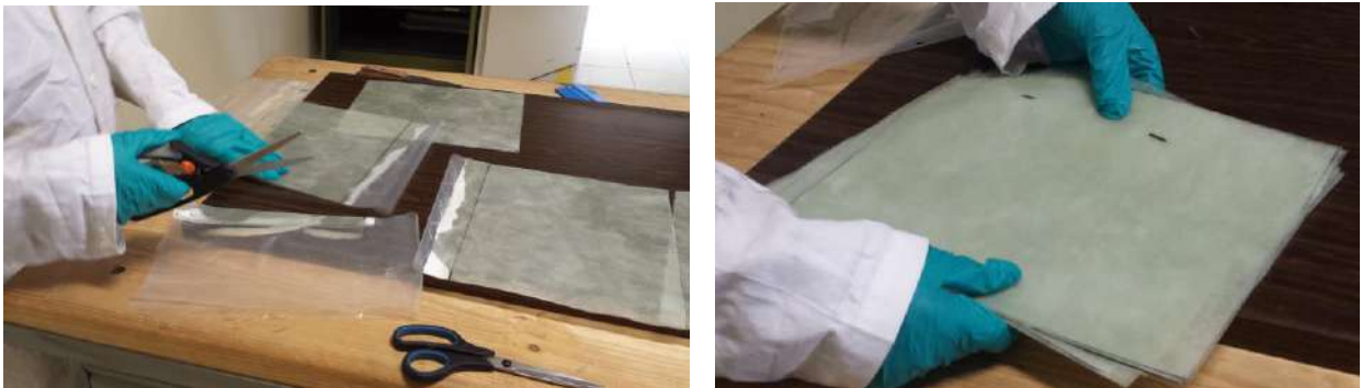
Figure 3.21: E-glass/Epoxy test specimen sizing
