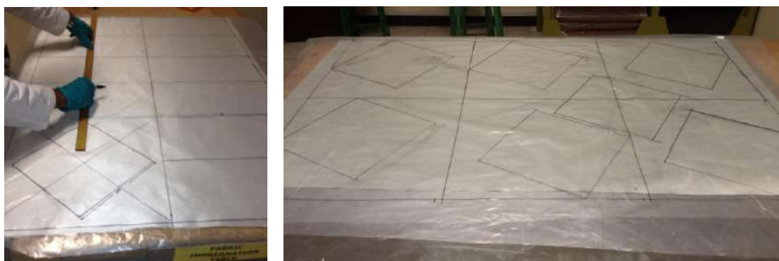
Figure 3.20: E-glass/Epoxy test specimen Layout
