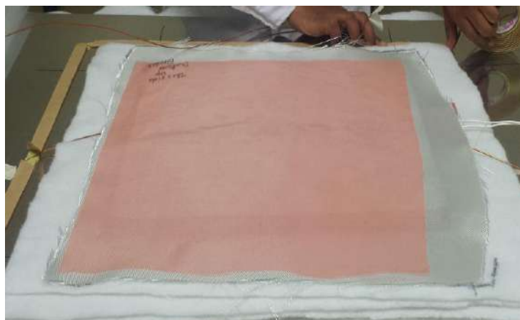
Figure 2.2 hand lay-up process
