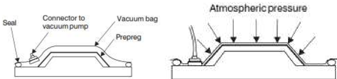
Figure 3.25: Application vacuum to E-glass/Epoxy
