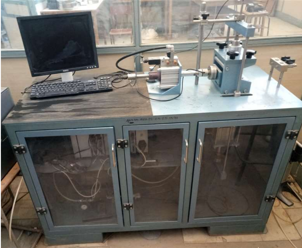
Figure 3.3: The cyclic shear testing apparatus at AAIT Geotechnical laboratory (See appendix J)
