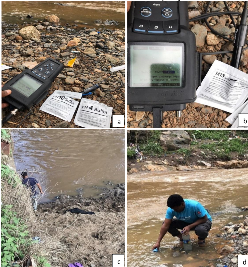
Figure 3-6 Physical parameter measurement at the field (a) & (b) instrument calibration (c) & (d) water sampling
