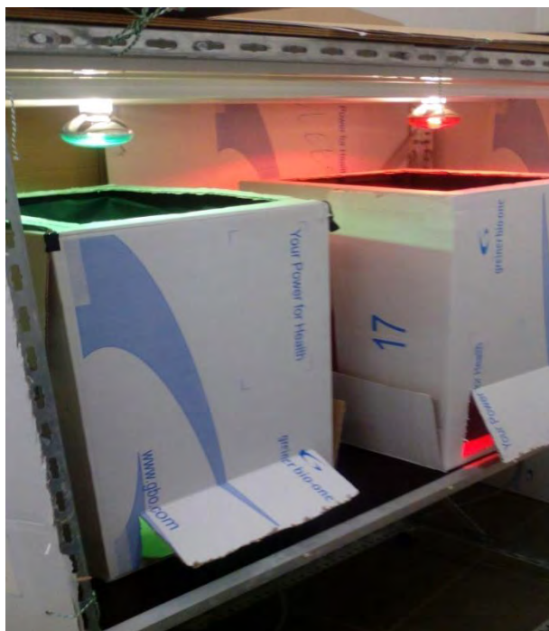
Figure 3.2 Illumination of raw beef slices under green and red color lamps inside of a black box
