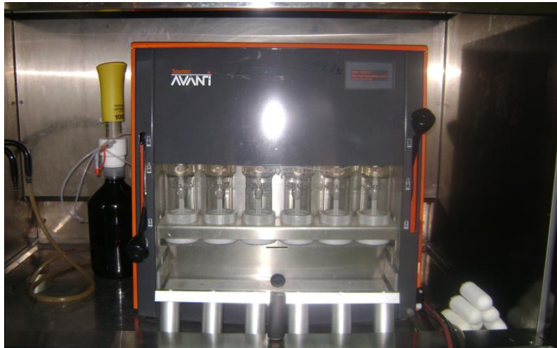
Figure 3.9 Soxtec Soxhlet fat extraction apparatus
