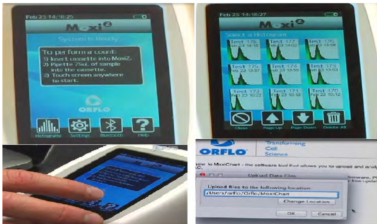
Figure 5-6: Connecting Moxi z with a PC via Bluetooth
