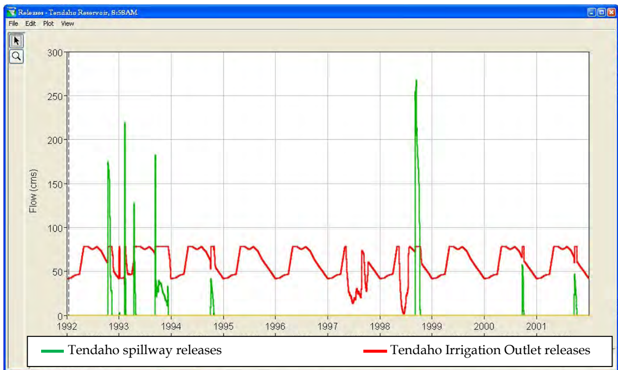
Figure 6.16. Reservoir releases for average level (4m) gate setting and Tendaho inflow.
