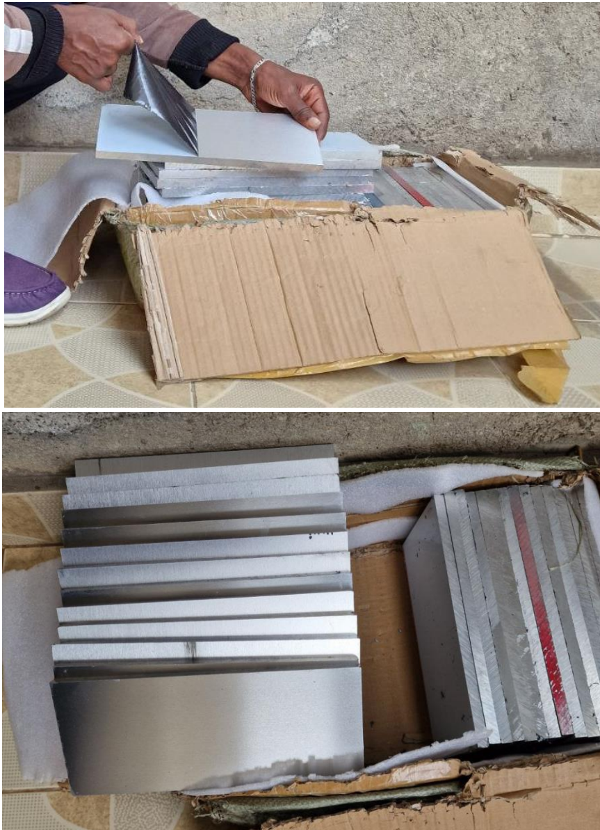
Figure 7: Unpacking and peeling of anti-oxidation film cover
