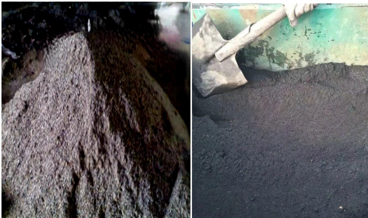
Figure 9: Coal, barium carbonate, sodium carbonate and calcium carbonate mixing
