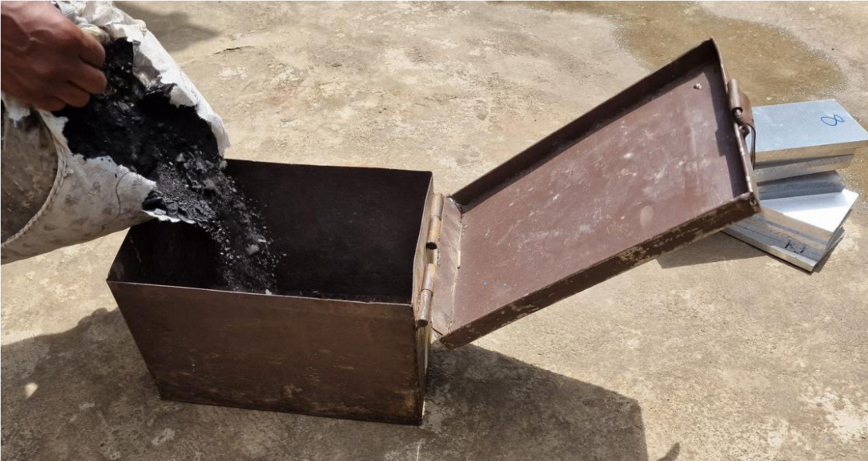
Figure 10: prefilling charcoal carbon mix in lockable steel container
