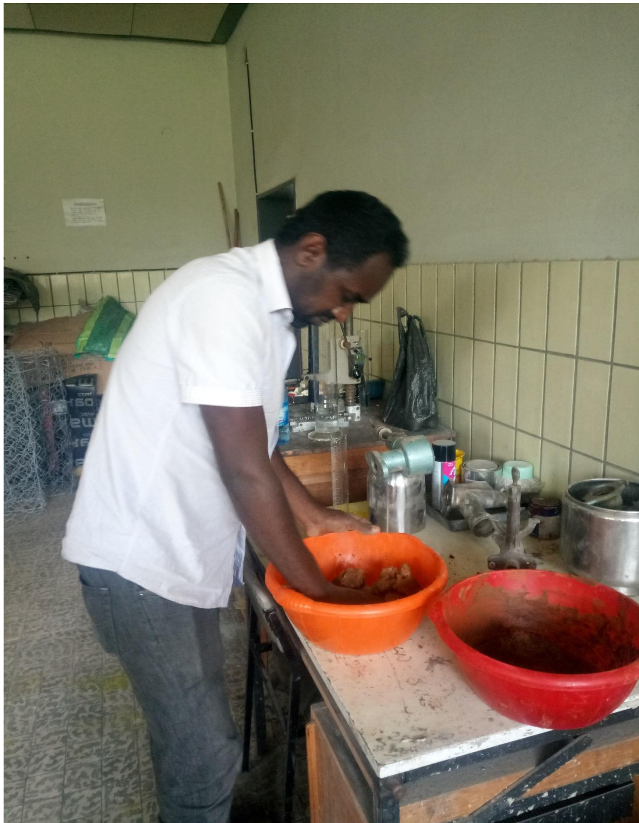
Pressing and mixing clay soil and sawdust to make ready for molding
