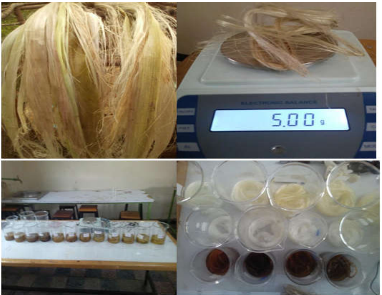
Fig 3.1 Banana fiber after soda treatment and bleaching with peroxide
