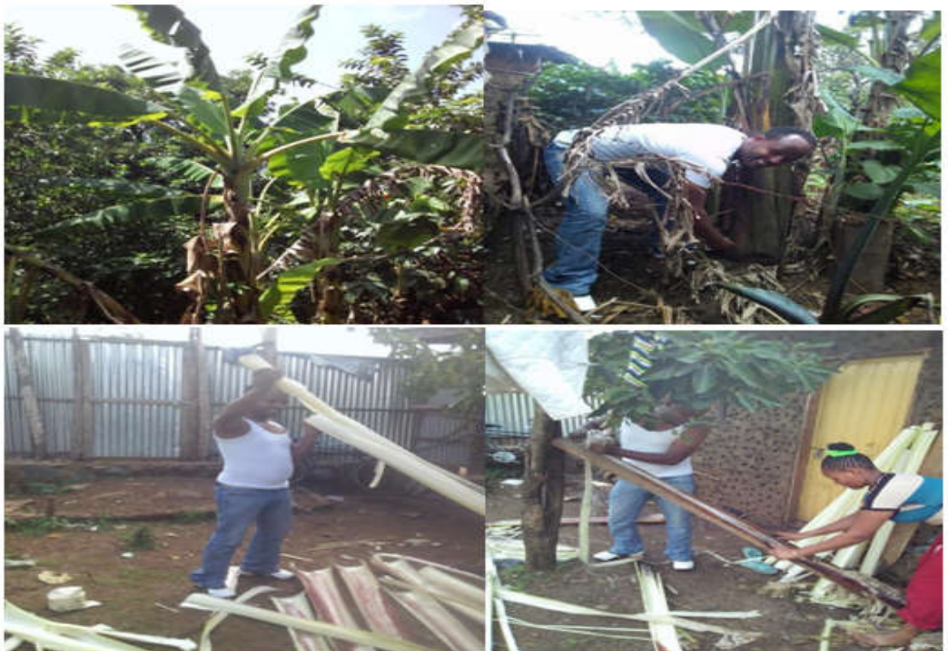
Fig.2.2extraction of banana fiber using manual method using iron ribbon
