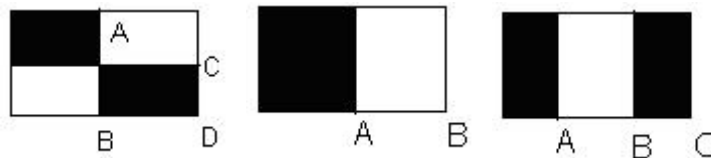
Figure 3-3 : Points used to calculate harr-like feature
