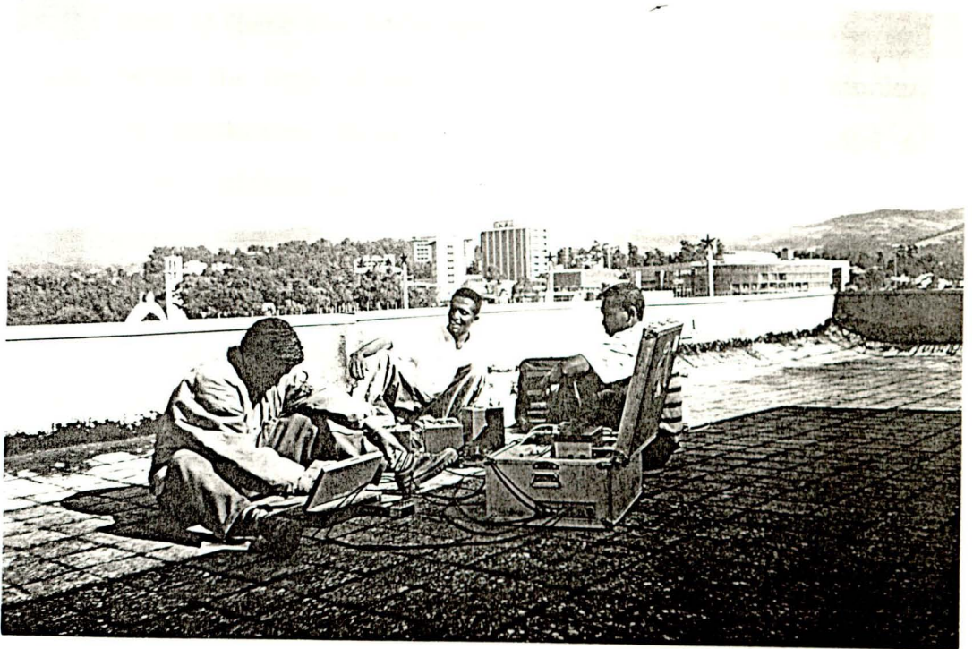
Fig.(2.8) Taking Microtremor Readings on top of Science and Technology Commission Building.
