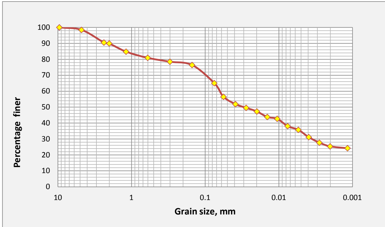
C24 Grain size distribution curve for TP6 at D=3.0m
