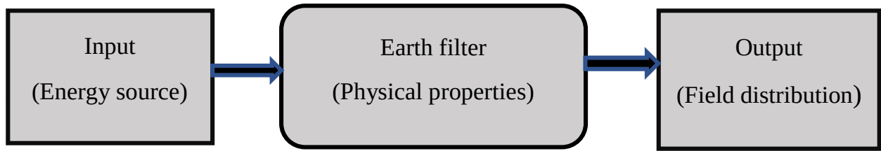
Figure 3.9 The main components of a geophysical remote sensing experiment
