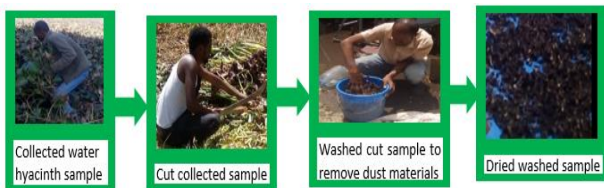
Figure 6-1. General Preparation of Water Hyacinth Biomass Sample
