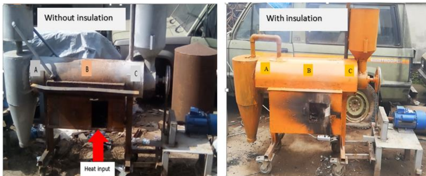
Figure 6-4. Reactor with and without ash insulation
