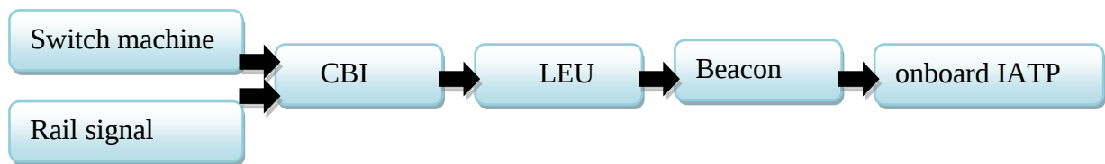
Figure 4-3 ITAP signaling subsystem reliability block model
