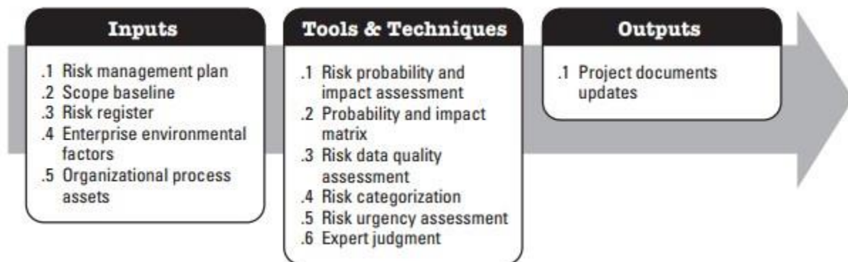
Figure 2.3 Qualitative risk Analysis: Inputs, tools & techniques, and outputs
