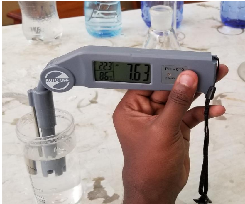
Figure 6: Measuring PH and temperature
