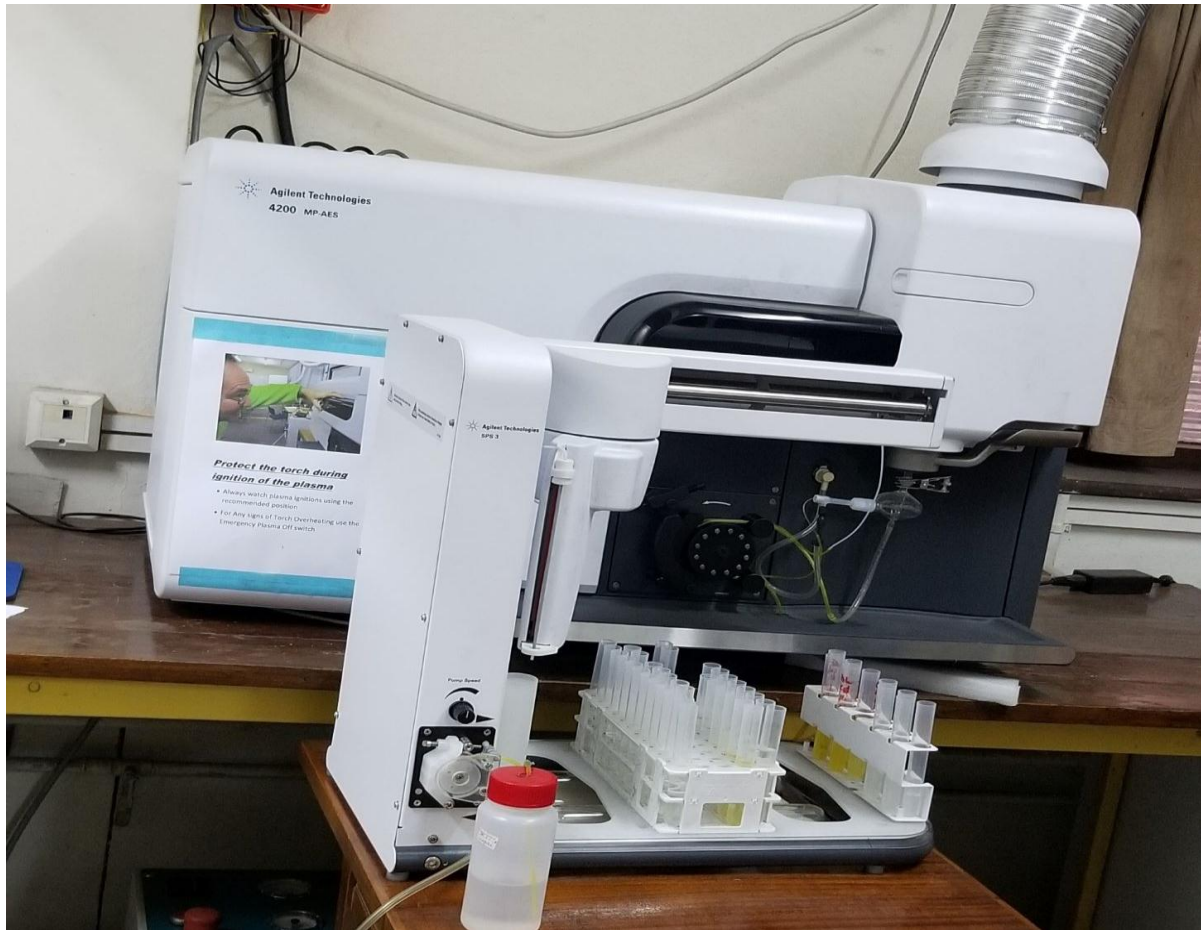
Figure 9: Agilent 4200 MP-AES measuring lead concentration
