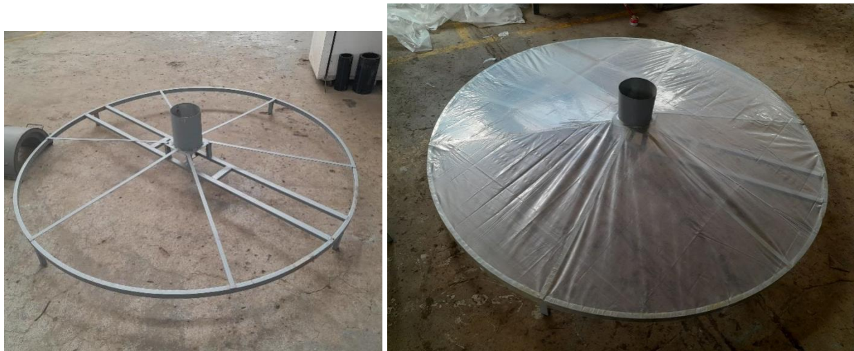
Figure 3.2 Collector with chimney support
