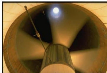
Figure 2.3 Turbine of the Manzanares prototype power plant [8]
