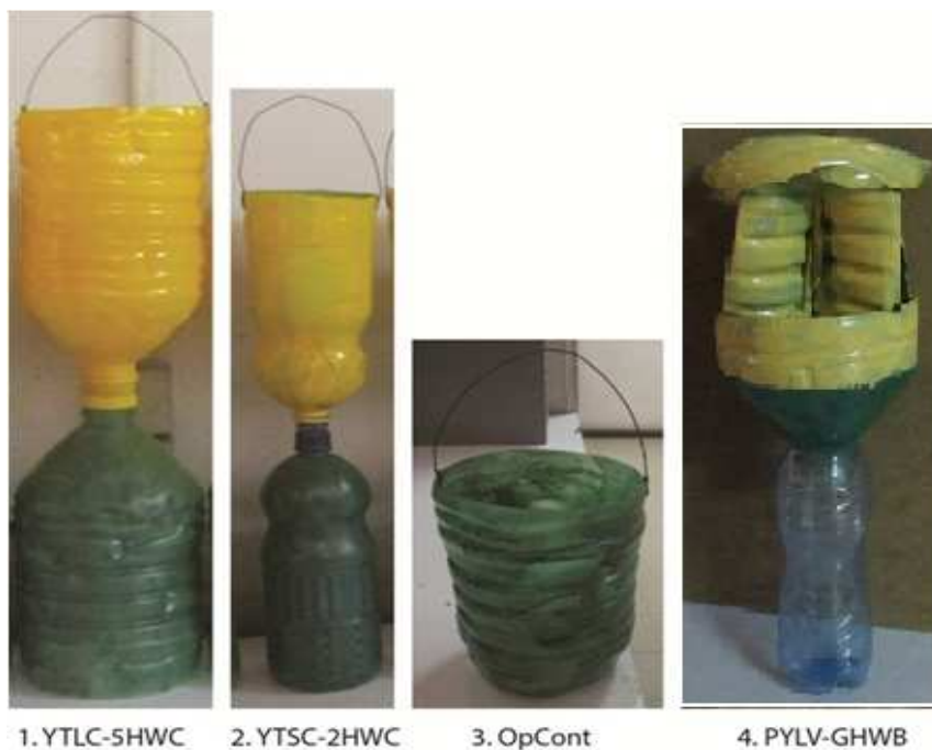
Figure 11. Four locally made traps tested for their effectiveness in catching and retaining adult P. interrupta in October 07-09, 2013. Trap 1, 2 and the vane and funnel design of trap 4 were the modification of green open container (trap 3), but different in size. The arrangement and description of traps are explained in table 4 above.
